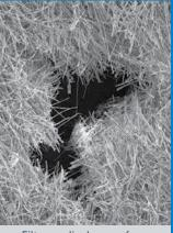
Filter media damage from Electrostatic Discharge (ESD).
